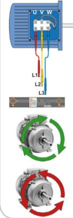
Connect the meter to the examined motor.
