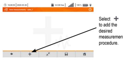
Select + to add the desired measurement procedure.
