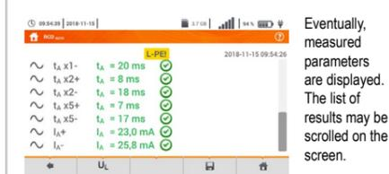
Eventually, measured parameters are displayed. The list of results may be scrolled on the screen.
