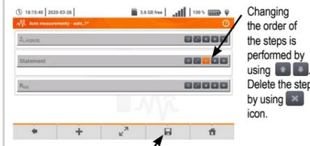
Changing the order of the steps is performed by using . Delete the step by using .
